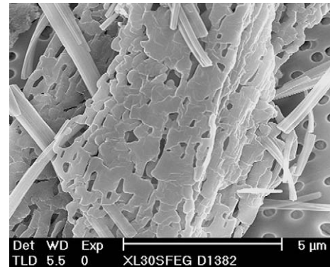
Fig. 4. SEM image of a smoothed surface grain and carbon rolled-up thin layers collected on the tile surface.
